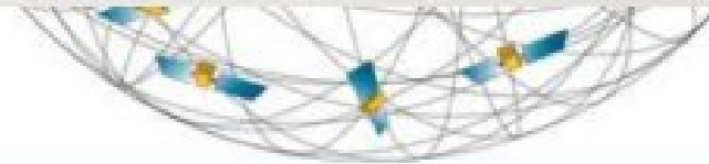
Figure 26 A GPS receiver uses signals from four of the 24 orbiting satellites to determine the receiver's location.
