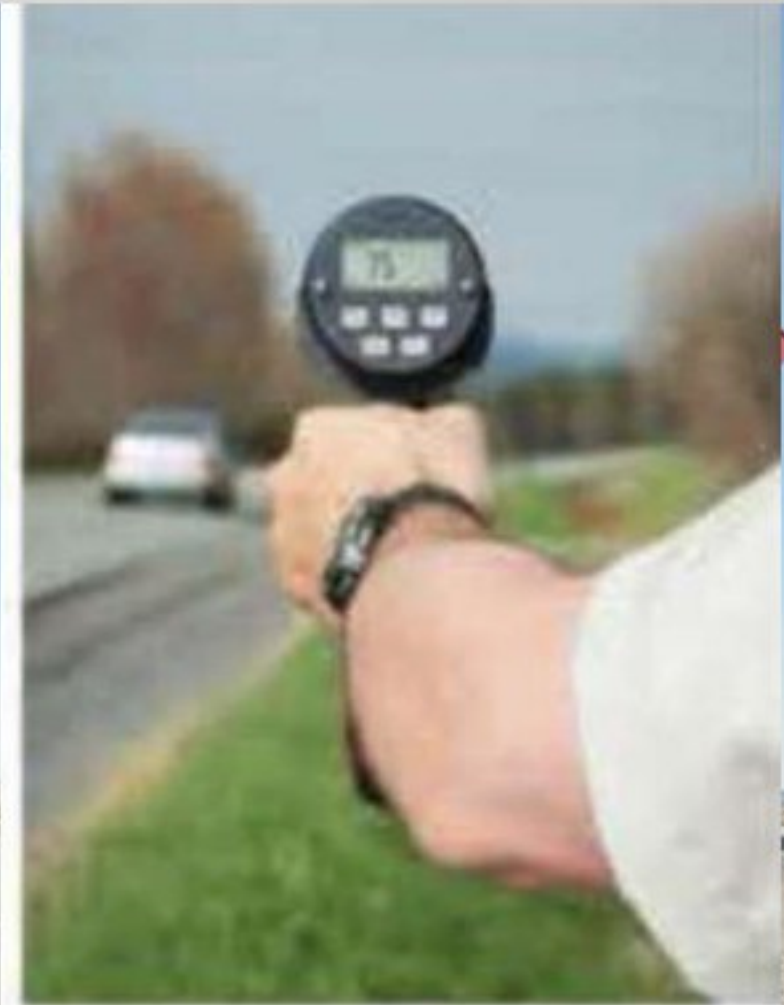
Figure 11 Police use radar guns to measure the speeds of motorists on highways. Radar guns function based on the Doppler effect.
