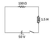
38-In the RL circuit shown in the figure, what is the current in the circuit at t= 5.2 ms?
