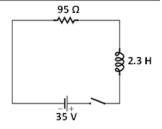
39-In the RL circuit shown in the figure a, what is the current in the circuit at t= 1.2 ms of opening the switch?
