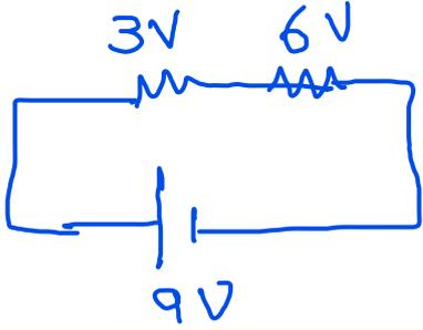
$$\frac{\Delta V_{\text{مصدر}}}{R_1 + R_2} = \frac{\Delta V_1}{R_1} = \frac{\Delta V_2}{R_2}$$
