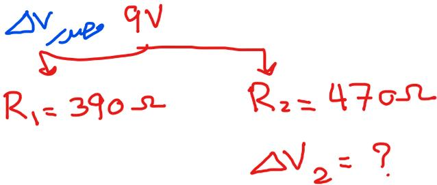
$$\frac{\Delta V_{\text{مصدر}}}{R_1 + R_2} = \frac{\Delta V_2}{R_2}$$
