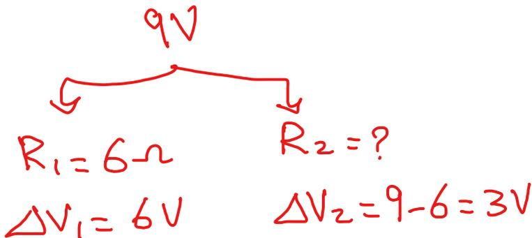
$$\frac{\Delta V_1}{R_1} = \frac{\Delta V_2}{R_2}$$
