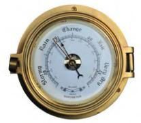
A barometer measures changes in atmospheric pressure and helps to predict whether it will be wet or dry.
