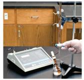
3. Measured volumes of the standard solution are added slowly and mixed into the solution in the beaker. The pH is read and recorded after each addition.
