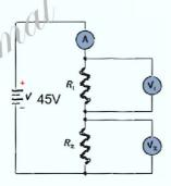
Suppose the circuit shown in Example Problem 1 has these values:  $R_1 = 255 \Omega$   $R_2 = 290 \Omega$ , and  $\Delta V_1 = 17 \text{ V}$ . No other information is available.
