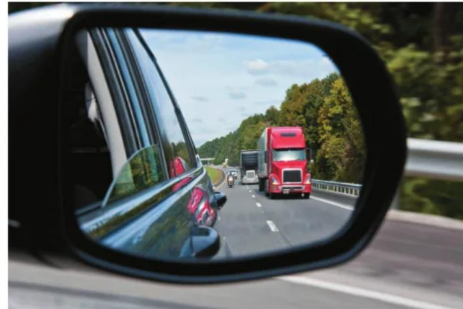
Figure 16 Images from convex mirrors are smaller than the object. This increases the field of view and decreases the driver's blind spot.
