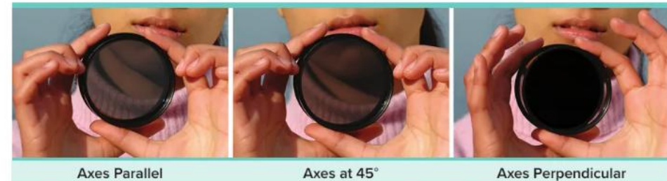
Figure 20 Polarizing filters with their axes parallel will allow the light with the same orientation to pass. With the polarizing axes at a 45^\circ angle, the filters allow some light to pass. If the axes of the filters are perpendicular, the second filter will block the light that has passed through the first filter.
