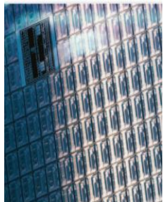
■ Figure 15.16 Sulfur hexafluoride is used to etch minute and sometimes intricate patterns on silicon wafers in the production semiconductor devices. Semiconductors are important components of modern electronic equipment, including computers, cell phones, and MP3 players.
