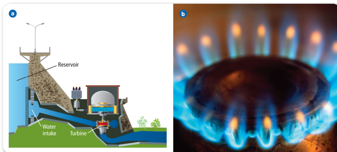
Figure 2 Energy can change from one form to another but is always conserved. In a , the potential energy of water is converted to kinetic energy of motion as it falls through the intake from its high position in the reservoir. The rushing water spins the turbine to generate electric energy. In b , the potential energy stored in the bonds of propane molecules is converted to heat.
