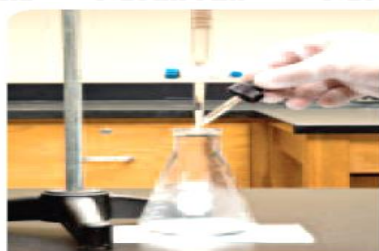
The buret contains the standard solution (0.1000M NaOH), and the flask contains 25.00 mL HCOOH solution along with a small amount of phenolphthalein indicator.
