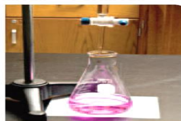
The end point of the titration is marked by a permanent, but very light, pink color. A careful reading of the buret reveals that 18.28 mL 0.1000M NaOH has been added.
