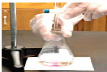
The standard solution is added slowly to the acid solution. The phenolphthalein indicator turns pink, but the color disappears upon mixing, until the end point is reached.
