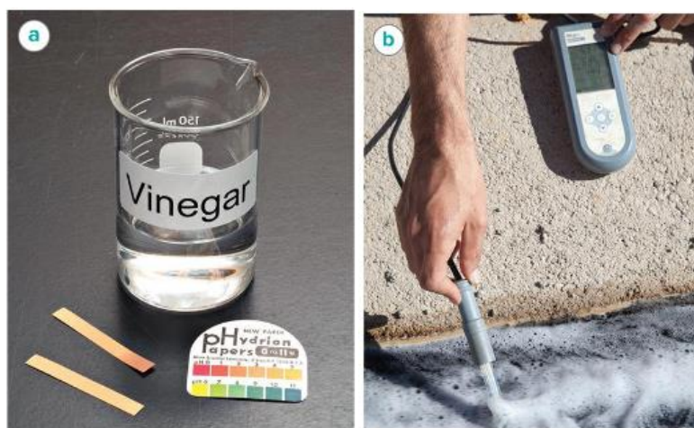
Figure 16 The approximate pH of a solution can be obtained by wetting a piece of pH paper with the solution and comparing the color of the wet paper with a set of standard colors as shown in a . The portable pH meter in b , which is being used to measure the pH of rain water, provides a more accurate measurement in the form of a digital display of the pH.
