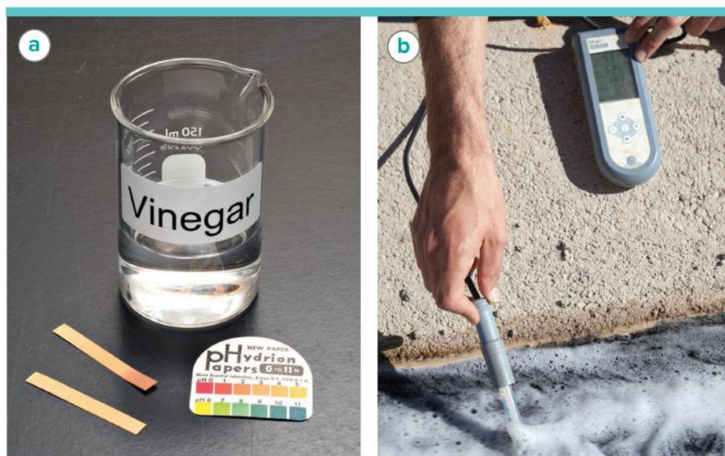
Figure 16 The approximate pH of a solution can be obtained by wetting a piece of pH paper with the solution and comparing the color of the wet paper with a set of standard colors as shown in a . The portable pH meter in b , which is being used to measure the pH of rain water, provides a more accurate measurement in the form of a digital display of the pH.
