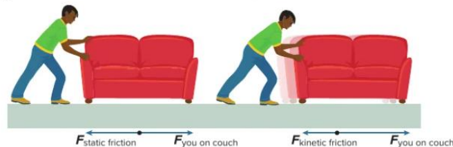
Figure 10 An applied force is balanced by static friction up to a maximum limit. When this limit is exceeded, the object begins to move.
