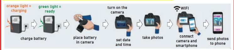
The diagram shows the different steps involved in using a digital camera for the first time.
