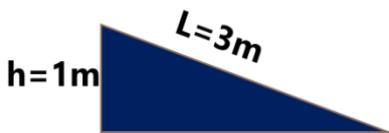
$$\begin{aligned} W &= \Delta E_p \\ &= mg(h_f - h_i) \\ &= 50 \times 9.8 (1 - 0) = 490 \text{ J} \end{aligned}$$
