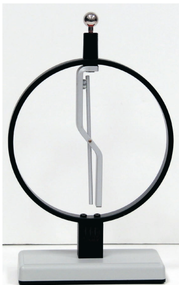
FIGURE 1.8 A typical electroscopes used in lecture demonstrations.
