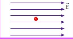
♣ A small positively charged object could be placed in a uniform electric field at position A or position B in the figure. How do the electric forces on the object at the two positions compare?
