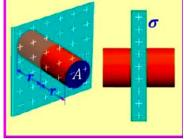
For an infinite conducting sheet with charge density  $\sigma > 0$  on each surface, we can find the electric field by choosing a Gaussian surface in the form of a right cylinder
