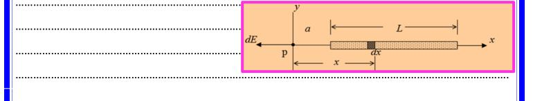
❖ Calculate the electric field at point p along the line that bisecting the wire
